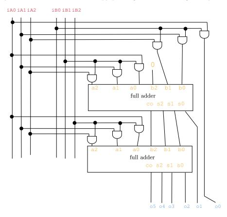
In this diagram, the blocks labelled 'full adder' are simply just copy-pastes (use structure blocks, clone, or worldedit!) of the adder you created in Part A. Just string those together with a few AND gates (which you can also copy over from your logical ALU section) and you should be good to go.
